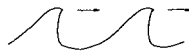
Fig.1. Schematic wave profile when wave breaking occurs. Matter at the very crest moves at the same speed as the wave profile.
